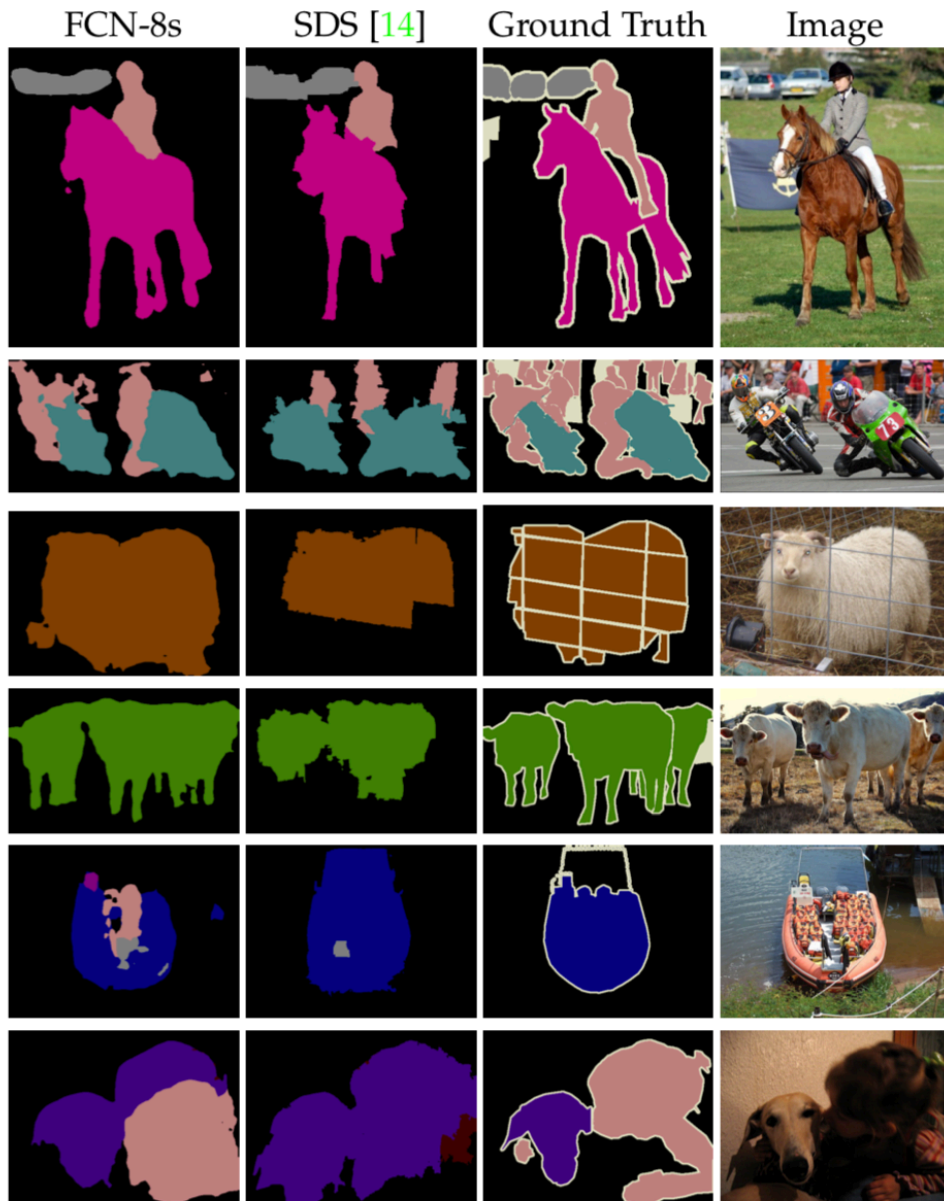
Fig. 6. Fully convolutional networks improve performance on PASCAL. The left column shows the output of our most accurate net, FCN-8s. The second shows the output of the previous best method by Hariharan et al. [14]. Notice the fine structures recovered (first row), ability to separate closely interacting objects (second row), and robustness to occluders (third row). The fifth and sixth rows show failure cases: the net sees lifejackets in a boat as people and confuses human hair with a dog.
